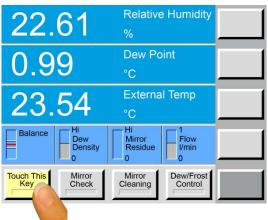
With the tip of your finger, press the center of the yellow highlighted key. After a successfully detection you will hear a click and the yellow Key switches position.
