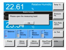
Press the *Ice Test* menu key. A window requests you to open the measuring head.
