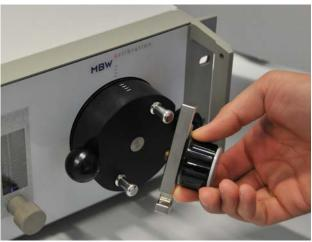
Once the clamp is removed, the black optical unit can be easily removed as shown. This part contains the optoelectronic components. An oval-shaped O-ring seals the measuring head. Gold contacts are located on the surface. Please avoid touching the surface of the optical unit with your fingers to avoid contamination of the contacts, the O-ring, the optical zone and the gas channel.
