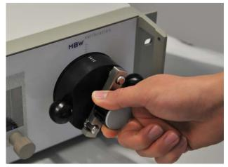
The measuring head of the dew point 373 is located on the right side of the front panel. To access the mirror or the other optical component to be removed, first, remove the measuring head clamp.
