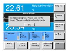
During Ice Test, the mirror rapidly cools to approximately -30 °C. Because the measuring head is open, humidity from the ambient air starts to condense on the mirror. This forms a frost layer on the mirror which can be increased if necessary by breathing on it. After reaching the low temperature and forming ice on its surface, the mirror begins to heat. As the temperature approaches 0 °C, the instrument will beep increasingly rapidly as the mirror gets closer to the ice-melt temperature.
