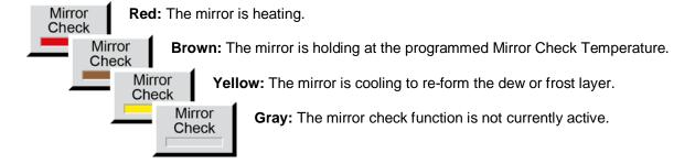
Once the system has re-established a dew or frost layer and become stable, the mirror check function is completed and the color indicator turns gray.
