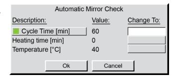
When the automatic mirror check is enabled, the *Mirror Check* key at the bottom of the screen shows a countdown timer indicating the time before the next automatic mirror check is performed. In the automatic mode, the mirror check may still be initiated manually by pressing the *Mirror Check* button.
