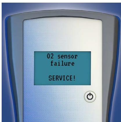
Fig. 3.2 – Sensor failure
