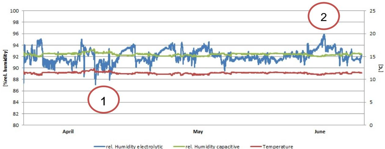
Peaks (1) and (2) originated from problems with the humidification/dehumidification installation, which was not detected by the building technology.
